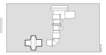
Connect ventilation hose to socket of breathing valve.
