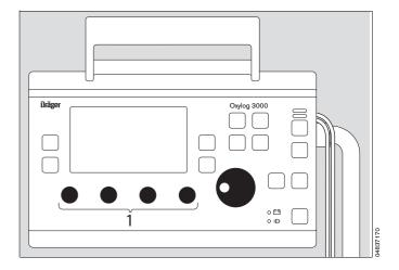
Oxylog 3000 successively activates the acoustic and visual alarm signals and prompts the operator to acknowledge each signal.
