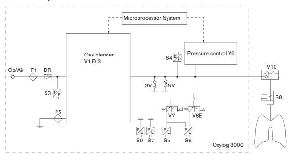
The variable pneumatic actuators in the Oxylog 3000 are controlled by the microprocessor system via digitized electrical test signals.
