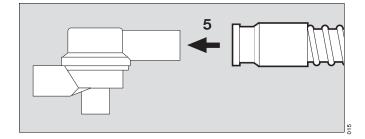
6 Fit the ventilation hose to the connector on the ventilator.
