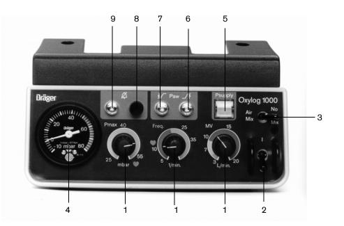
1 Three rotary control knobs are located in the middle of the front panel for setting the upper alarm limit for airway pressure (»Pmax«), the ventilation rate (»Freq.«) and the minute volume (»MV«).
