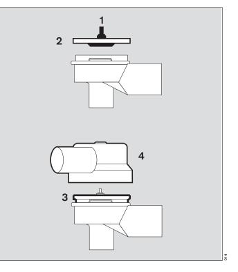
**5** Fit the ventilation hose to the inspiration connector of the ventilation valve.
